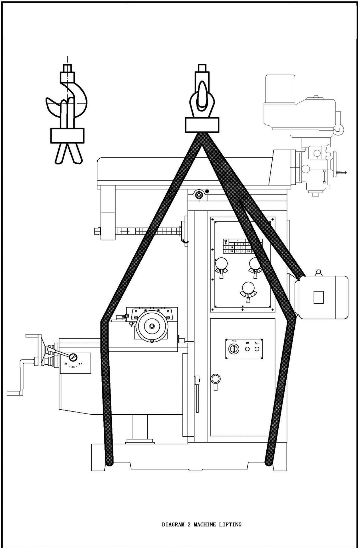
DIAGRAM 2 MACHINE LIFTING
